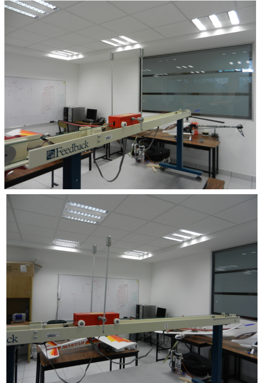
Fig 2: Inverted pendulum system used for the experiments
