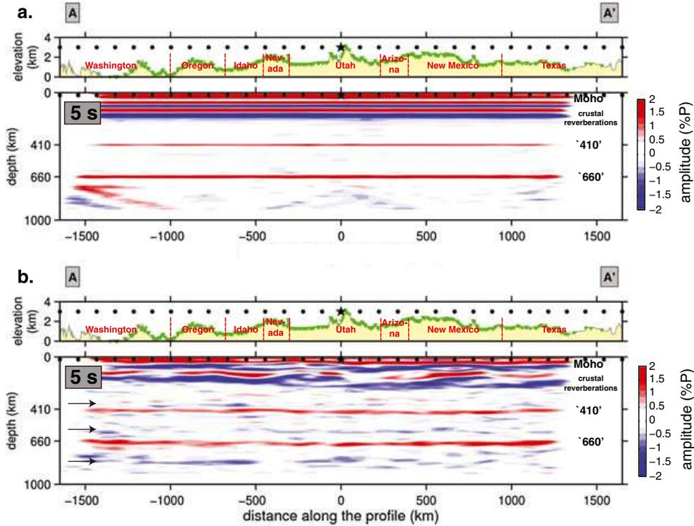
**Figure 3.** CCP stacked sections from USArray P-to-S receiver functions. Positive amplitudes are shown in red and negative amplitudes in blue. (a) A-A' section obtained from synthetic data computed with IASP91. The data are low-pass filtered at 5 s period. (b) Same section but for observed data. Black arrows indicate the depths of signals of specific interest.
