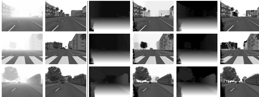
Fig. 3. Results on three images of the synthetic FRIDA3 stereo image database. First column: foggy left images. Second column: same scene without fog. Third and fourth columns: disparity maps obtained using stereo reconstruction without fog and restored images using these disparity maps. Fifth and sixth columns: disparity maps with the proposed method and associated restored images.
