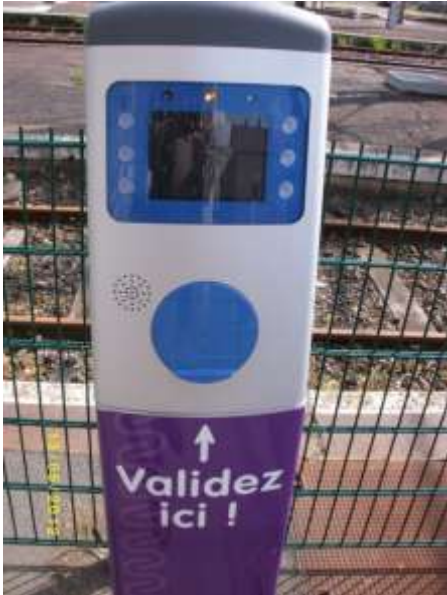
Figure 14 : smart card terminal for validation of tickets in Armentières railway station (photo L'Hostis-Belibi)
