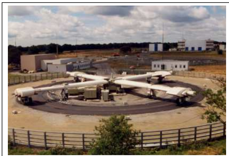
Figure 1 - LCPC Carousel and fatigue test track.
