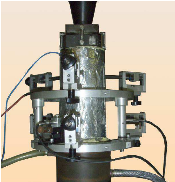
Figure 3: Extensometer and test setup for cyclic loadings on unconfined specimens. This setup was used to validate BTJASPE.
