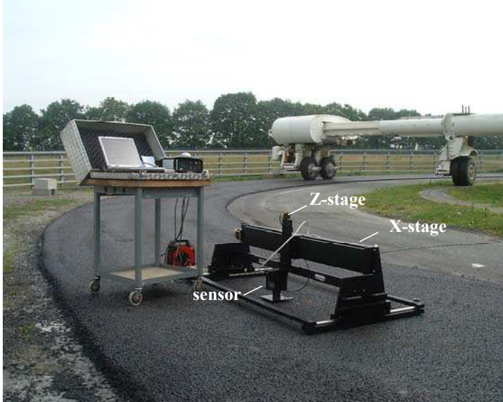
FIGURE 8 Laser device for profile measurement and location of profiles.
