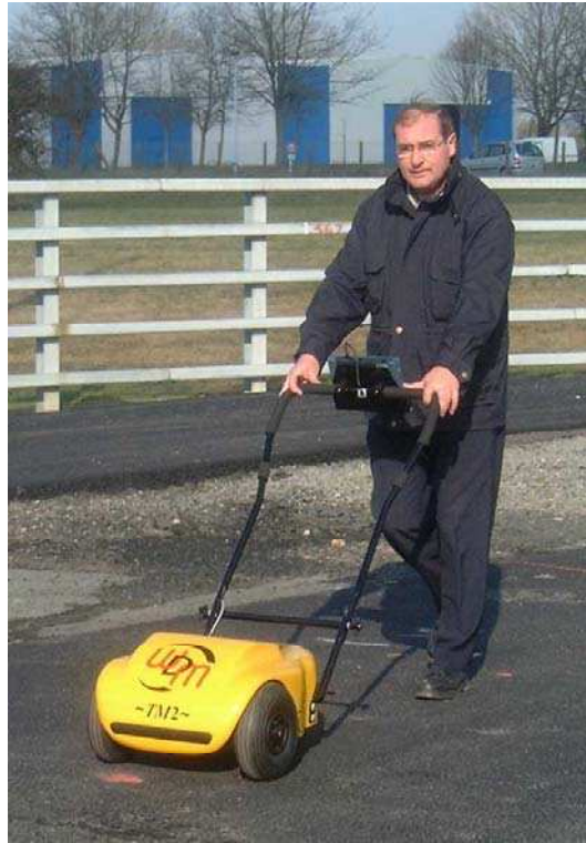
FIGURE 7 Mobile device for mean profile depth measurement.
