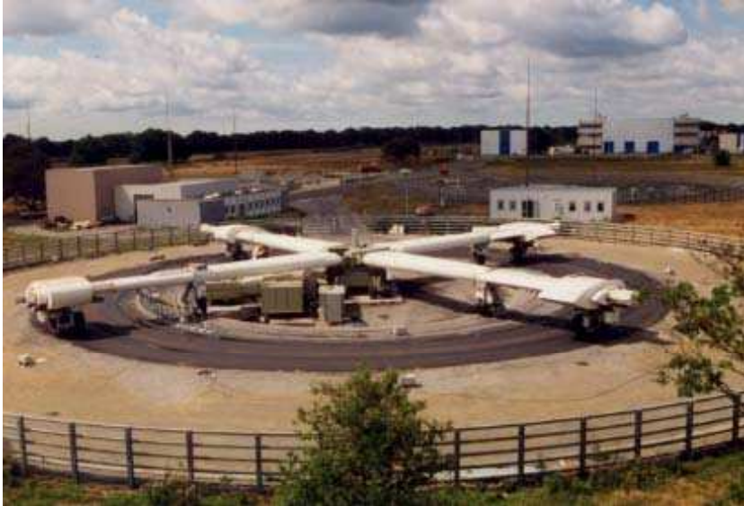
FIGURE 2 LCPC Carousel and fatigue test track.
