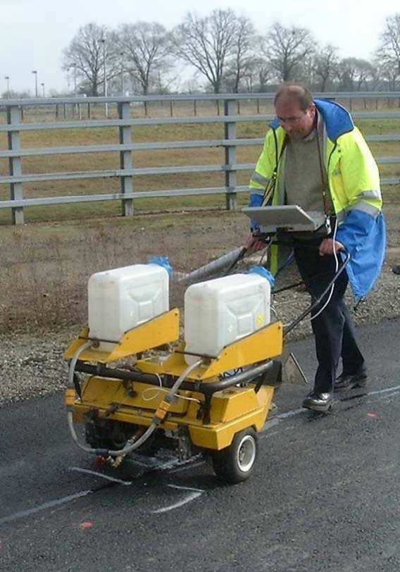
FIGURE 10 Mobile device for dynamic friction measurement.
