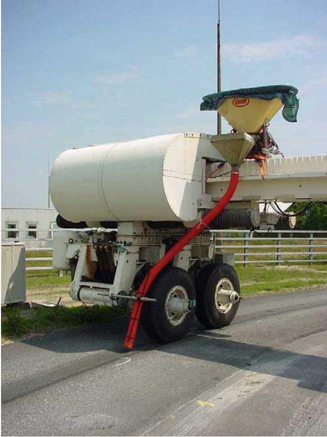
FIGURE 5 Set up employed for spreading of abrasive.
