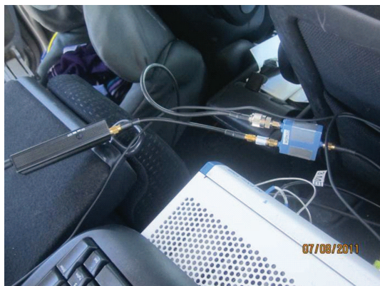
FIGURE 18: Handheld jammer signal combined with GPS signal via cabling and connected to the logging system.
