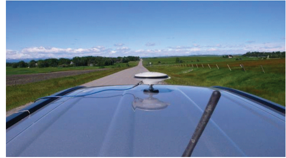
FIGURE 15: NovAtel 702 GG antenna mounted on the vehicle rooftop.
