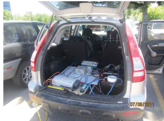
FIGURE 16: Tactical grade IMU (Honeywell HG1700) shown inside the vehicle.
