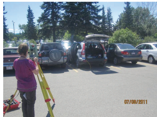
FIGURE 19: Lever arm surveying using Leica TCR705 reflectorless total station.
