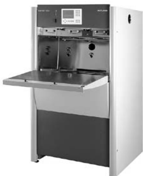
17 a) 18 FIGURE 5 Ageing test (a: weatherometer for accelerated test; b: specimens artificially 19 and naturally aged).
