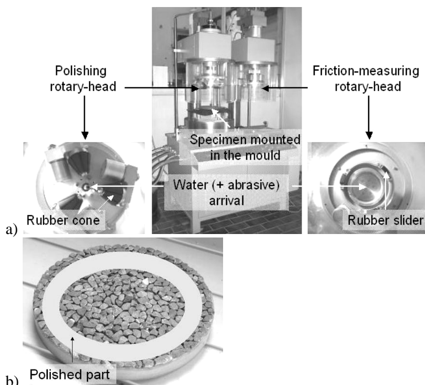
FIGURE 1 Wehner/Schulze machine (a: view of the machine and the two rotary heads; b: specimen and illustration of the polished part).
