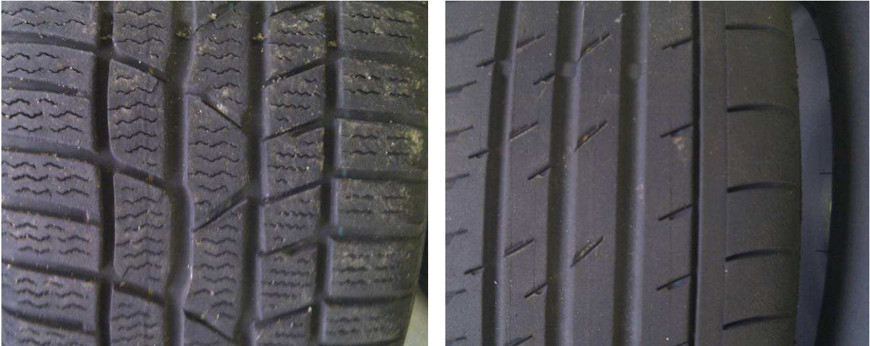
Figure 13 – Pattern differences between winter (left) and summer (right) tires
