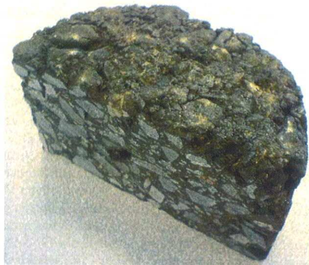
FIGURE 7 Mix manufactured with microalgae oil, using oedometric compaction system.
