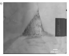
Fig. 5. TEM observations of (a) a vitreous triple point (white triangle) in material 4 (its composition is close to that of anorthite) and (b) an anorthite crystallized triple point (grey speckled) in material 26.
