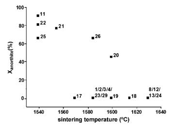
Fig. 10. Crystallization rate of anorthite  $X_{\text{anorthite}}$  as a function of the sintering temperature.
