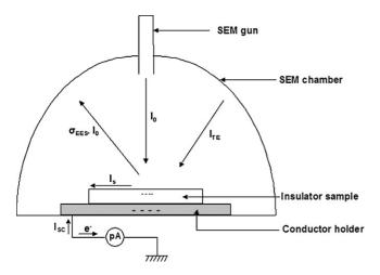
Fig. 1. Experimental set-up for ICM and SEMME measurements.
