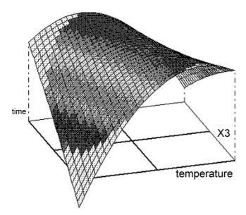
Fig. 2. Response surface of  $E_b$  versus soaking conditions (temperature and time); others parameters are at there median values: attrition time 15 min, additives content: 4.13 wt.%.
