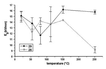
Fig. 6. Breakdown strength versus temperature for materials 26 (with anorthite crystals) and 29 (without anorthite crystals).
