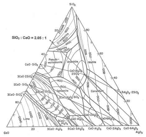
Fig. 12. Phase diagram of the ternary system Al<sub>2</sub>O<sub>3</sub>-CaO-SiO<sub>2</sub>.<sup>24</sup>
