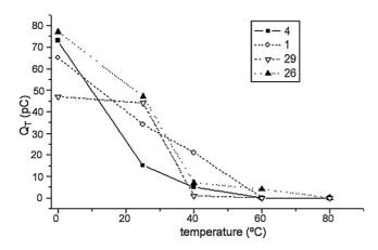
Fig. 7. Stabilised trapped charge amount  $Q_t$  as a function of the temperature for the four materials 4, 1, 29 and 26—injected charge amount  $Q_i = 300 \,\mathrm{Pc}$ .
