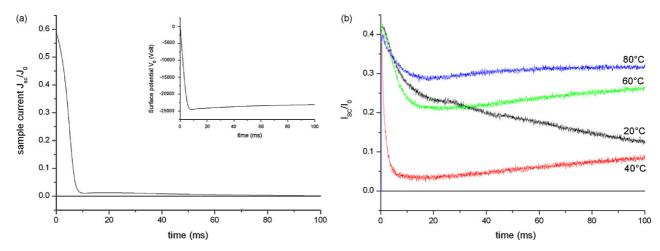
Fig. 8. Evolution of the sample current  $I_{SC}$  as a function of irradiation time for the material 29: simulated curve with the simultaneous variation of the surface potential (a) and influence of the temperature on  $I_{SC}$  experimental curves (b).
