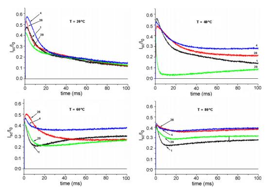
Fig. 9. Evolution of the induced sample current I<sub>SC</sub> as a function of irradiation time for the four materials 4, 1, 29 and 26 at different temperatures.
