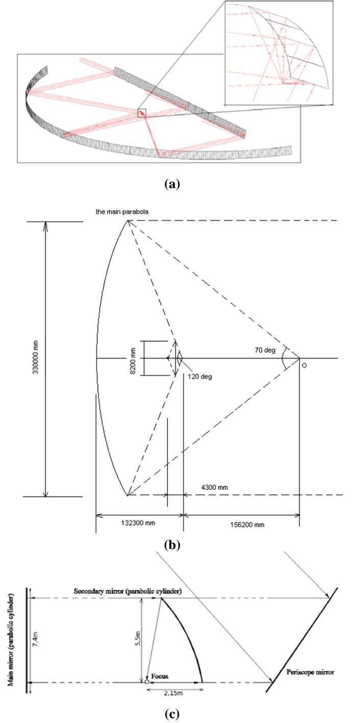
Fig. 1. The primary and secondary reflectors of the RATAN-600 radiotelescope (south sector): (a) Schematic 3D view; (b) Horizontal cut; (c) Vertical cut.
