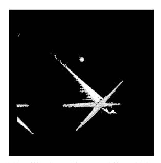
**Fig. 11.** Diamond-like region around the transverse stitching yarn (size in voxels:  $910 \times 910 \times 180$  and resolution: 5.5 µm).
