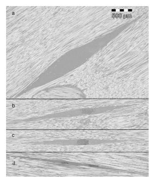
**Fig. 12.** Effects of diameter and tension of yarns on openings within plies: (a) yarn B; (b) loose yarn A; (c) tight yarn A; and (d) yarn C (2D destructive micrographies).
