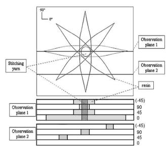
Fig. 6. Schematic view of resin-rich region in a quasi-isotropic multiply.
