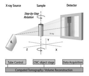
Fig. 9. X-ray microtomography equipment [7].
