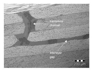
Fig. 1. Transverse channels and interlayer gaps (through-the-thickness section).
