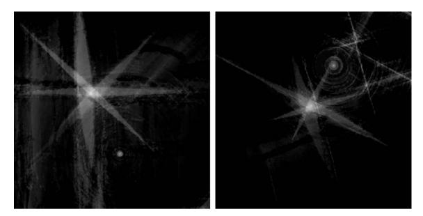
Fig. 16. Examples of two projections of resin-rich regions from two different samples.
