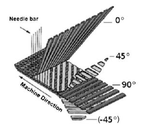
Fig. 3. NCF structure: ply assembly of a quasi-isotropic multiply [1].
