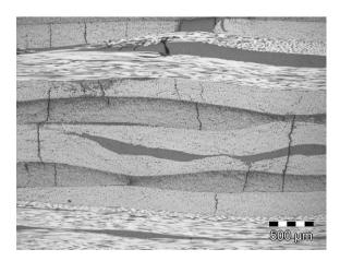
Fig. 17. Hygrothermal microcracks from cyclical loading.
