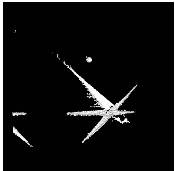
Fig. 11. Diamond-like region around the transverse stitching yarn (size in voxels: 910 \times 910 \times 180 and resolution: 5.5 \mu\text{m} ).
