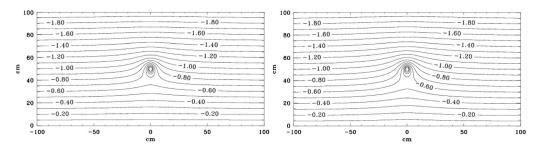
**Figure 4.** Equipotential contours around the SDA electrode at 0 V in (left) the model without cable and in (right) the model with coaxial bootstrapped cable.
