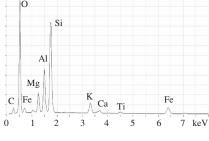
**Figure 5.** (left) Image of a soil sample from the playa, made with a scanning electron microscope (SEM). Energy of the SEM electron beam was fixed at 2 keV. The scale shown is in 10  $\mu$ m increments. (right) A typical energy-dispersive X-ray spectrum of the soil sample. Energy of the SEM electron beam was fixed at 15 keV.
