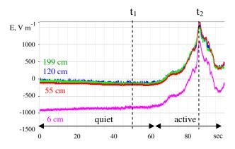
**Figure 6.** Vertical component of electric field measured by FM sensors at four heights. Positive/negative values correspond to upward/downward electric field.
