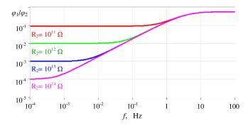
**Figure 3.**  $\varphi_1/\varphi_2$  versus frequency for various values of the  $R_2$  resistance.  $R_r$  is fixed at 10G $\Omega$ .
