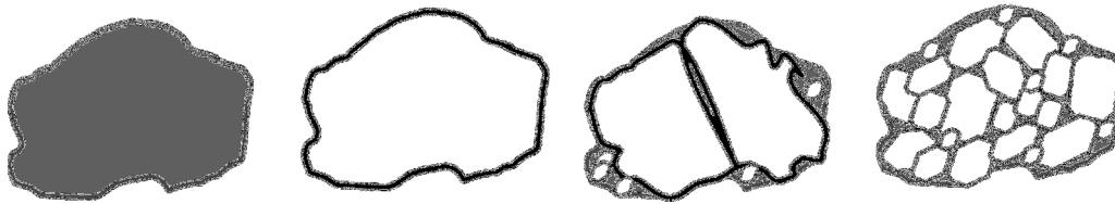
Figure 1: From the outside of a RA particle it is difficult to suggest its composition, which can be very different (From left to right: RA particle from the outside, cross sections of possible compositions of a RA particle: single coated aggregate, two major aggregates with some mastic, conglomerate of small aggregate particles and mastic)
