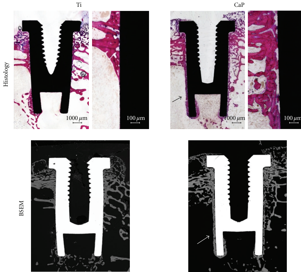
FIGURE 6: Micrographs showing the osteointegration of bare titanium- (Ti-) and calcium phosphate- (CaP-) coated implants after implantation in femoral condyles of rabbits for 4 weeks. Note the direct bone apposition on CaP-coated implants (arrows) on both histology (basic fuchsin, toluidine blue staining) and back-scattered electron microscopy (BSEM) images.
