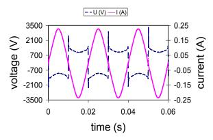
Figure 2. Variations of the voltage and current as a function of the time, inlet liquid volume ethanol/water ratio = 0.23.
