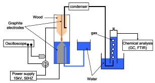
Figure 5: Schematic of experimental reactor
