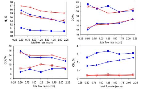
**Figure 3**.  $H_2$ , CO, CO<sub>2</sub> and CH<sub>4</sub> concentrations vs. the inlet total flow rate. Open symbols: methanol+water mixtures; full symbols: ethanol+water mixtures. Alcohol/water volume ratios: square symbols: 0.23; diamond symbols: 0.61.
