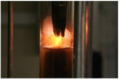
**Figure 6**: photography of the discharge between electrodes.
