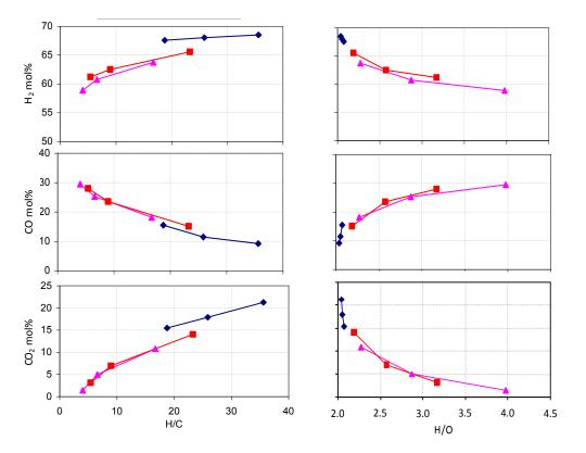
**Figure 4.**  $H_2$ , CO, CO<sub>2</sub> mol% vs. inlet H/C and H/O ratios.  $\blacktriangle$  methanol+ $H_2$ O;  $\blacksquare$  ethanol+ $H_2$ O;  $\blacklozenge$  phenol+ $H_2$ O.
