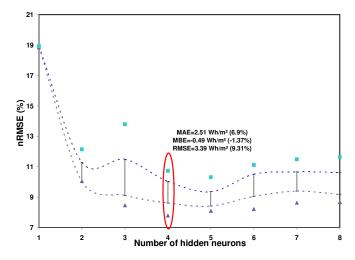
Figure 5. nRMSE evolution vs. the number hidden neurons for the ANN model with five inputs.
