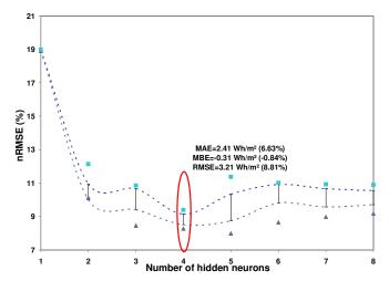
Figure 6. nRMSE evolution vs the number hidden neurons for the ANN model with four inputs.
