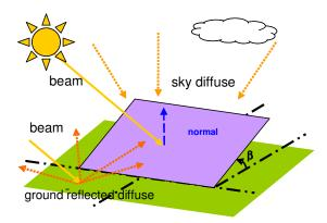
Figure 1. Solar radiation on a tilted surface
