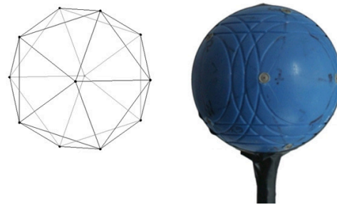
Figure 2: Second order ambisonics microphone. Left, sketch of 12 sensors placed in dodecahedron. Right, the prototype developed at Orange Labs.
