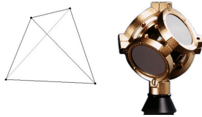
Figure 1: SoundField microphone. Left, sketch of a regular tetrahedron. The capsules are placed on each side. Right, SoundField microphone from Farrar’s work [20, 21].
