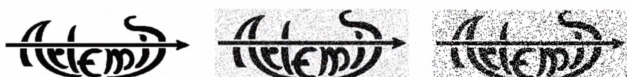
Figure 3: The original ARTEMIS (left) binary logo recovered after transcoding (middle) and geometric attacks (right).
