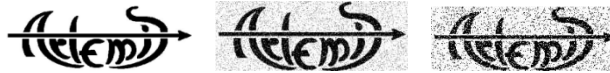
Figure 5. The original ARTEMIS (left) binary logo recovered after transcoding (middle) and geometric attacks (right).
