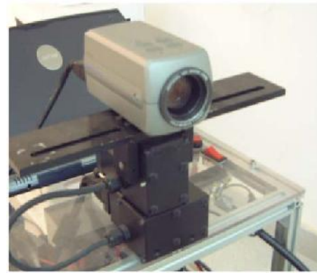
Fig. 2 The camera and pan-tilt unit used to take the images
