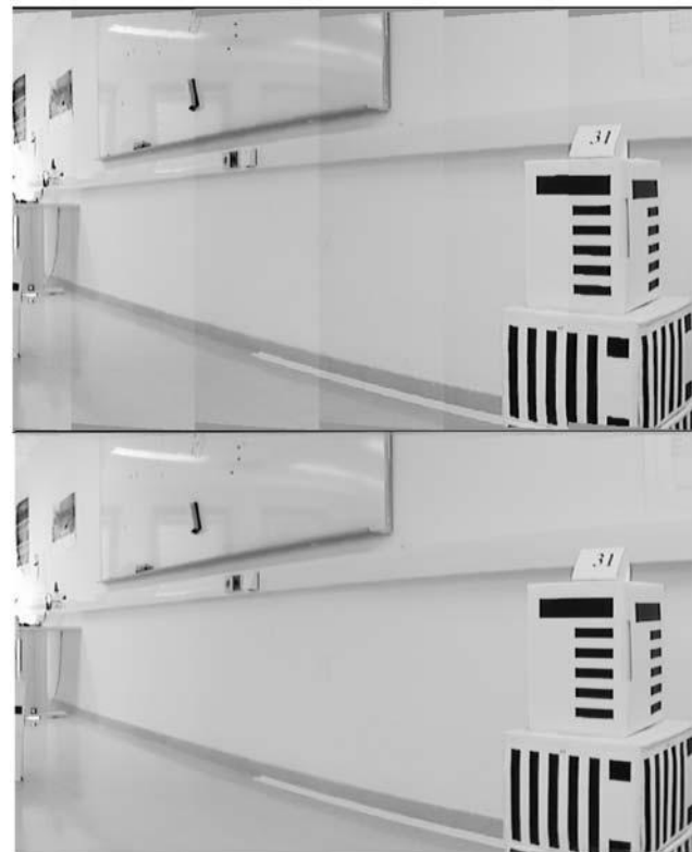
Fig. 3 Intensity jumps between successive images caused by automatic camera gain ( top ). Applying linear blending solves the problem ( bottom )
