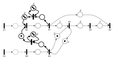
Fig. 2 A TEG (thin lines) merged with a realization of its controller (thick lines) and the (external) reference inputs (dotted lines).
