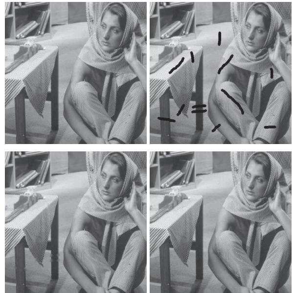
Fig. 3. Inpainting on barbara image using a window 21 and patch 5. From left to right, the original image, the corrupted image, the result of a local inpainting and our nonlocal inpainting result.
