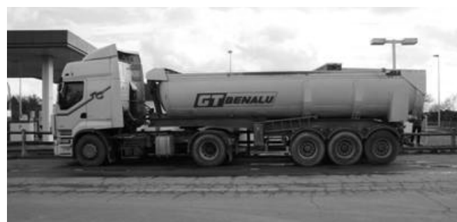
Figure 18. 44 ton heavy vehicle with tridem rear axle system, wheelbase = 112 cm.
