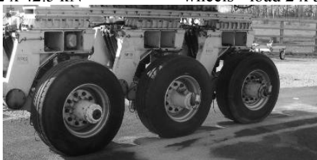
Tridem axle with single wheels - load 3 x 42.5 kN
