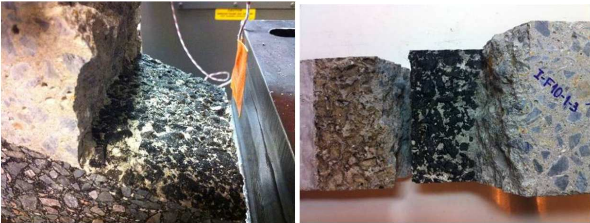
Figure 7. Visual debonding fracture aspect of Type I specimen: a) I-PT-2-3 b) I-PT-1-3
