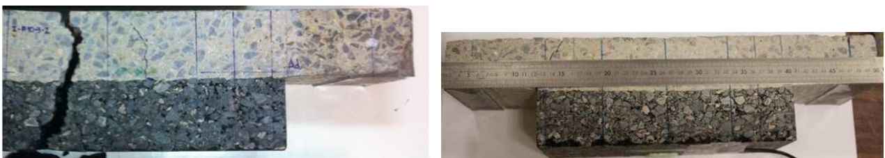
Figure 8. Bending parasite failures at the: a) Middle of the beam (I-PT-3-2) b) Edge of layer 2 due to non regular thickness of layers (Type I-PT-2.1 example)
