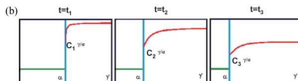
**Fig. 10.** (a) Expected evolution of the tie-lines during austenite growth at  $755^\circ\text{C}$  for Fe-0.15C-0.215Si-1.9Mn-0.195Cr. The calculations were done with the THERMOCALC software. The red circle indicates the nominal composition and the equilibrium tie-line is the solid red line marked  $t_2$ . (b) Schematic showing the expected evolution of the carbon profiles during austenite growth at  $755^\circ\text{C}$  for Fe-0.15C-0.215Si-1.9Mn-0.195Cr.
