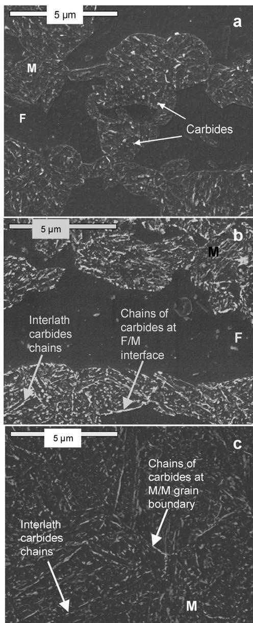
**Fig. 7.** SEM micrographs showing the evolution of different microstructures with tempering. Picral etching. a)  $T_Q = 755^\circ\text{C}$ ,  $T_T = 230^\circ\text{C}$ , b)  $T_Q = 755^\circ\text{C}$ ,  $T_T = 460^\circ\text{C}$ , c)  $T_Q = 810^\circ\text{C}$ ,  $T_T = 460^\circ\text{C}$ .
