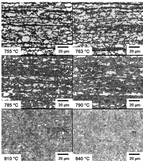
**Fig. 2.** Optical micrographs of the as-quenched samples. Picral and Metabisulfite etching: the dark-etching phase is martensite, the white-etching phase is ferrite.
