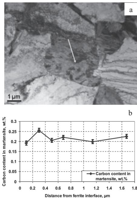
Fig. 6. TEM image of a martensite island in as-quenched  $T_Q = 755^\circ\text{C}$  sample (a) and (b) EELS C concentration measurements taken from the ferrite interface to the centre of the island following the arrow.
