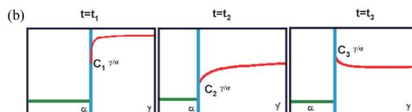
**Fig. 11.** (a) Expected evolution of the tie-lines during austenite growth at  $790^\circ\text{C}$  for Fe-0.15C-0.215Si-1.9Mn-0.195Cr. The calculations were done with the THERMOCALC software. The red circle indicates the nominal composition and the equilibrium tie-line is the solid red line marked  $t_2$ . (b) Schematic showing the expected evolution of the carbon profiles during austenite growth at  $790^\circ\text{C}$  for Fe-0.15C-0.215Si-1.9Mn-0.195Cr.
