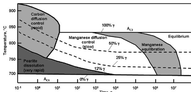
**Fig. 9.** Austenite growth diagram for Fe-0.12C-1.5Mn-0.24Si steel.<sup>29)</sup>
