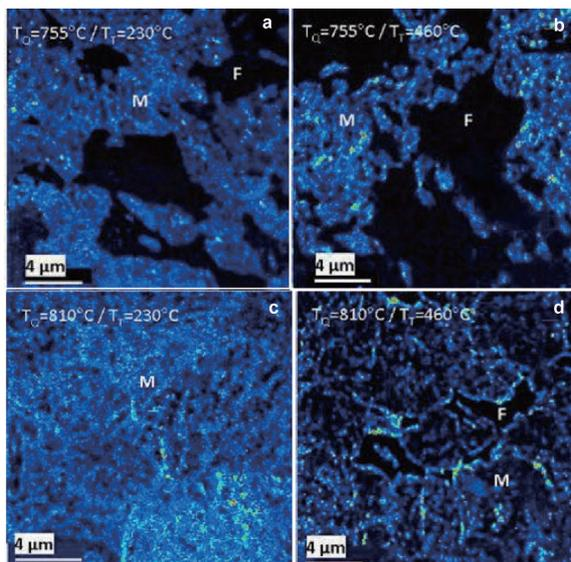
**Fig. 8.** Qualitative SIMS carbon maps from samples quenched at  $T_Q = 755^\circ\text{C}$  (a, b) and  $T_Q = 810^\circ\text{C}$  (c, d) and tempered at  $230^\circ\text{C}$  (a, c) and  $460^\circ\text{C}$  (b, d). The carbon content increases from black to red.
