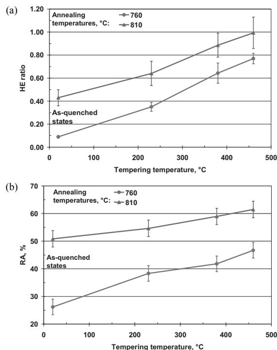
Fig. 13. (a) HE ratio evolution with tempering temperature for 760°C and 810°C annealing temperatures. (b) Variation in the reduction of area (RA) with tempering temperature for 760°C and 810°C annealing temperatures.
