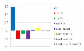
Fig. 4. The diagram effects for the model (from left to right), M is the average lifespan while the other terms are the stress effects; results are in the same order as in Table V i.e. first M, then log(V), etc.
