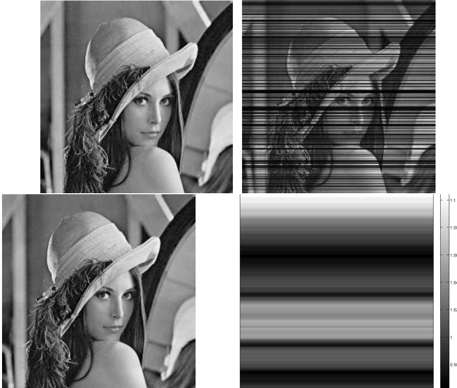
FIG. 1.2. An example involving a multiplicative noise model. From left to right. Original image - Noisy image. It is obtained by multiplying each line of the original image by a uniform random variable in [0.1, 1] . SNR=10.6dB - Denoised using the method proposed in [8] on the logarithm of the noisy image. SNR=29.1dB - Ratio between the original image and the denoised image. The multiplicative factor is retrieved accurately.
