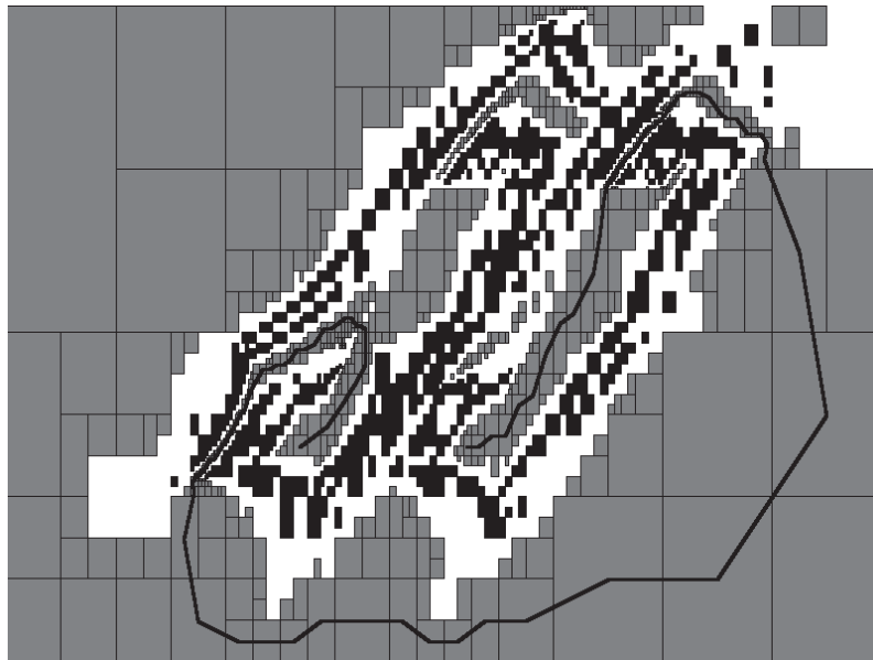
Figure 9: Paving and path generated by FEASIBLEPATH2.
