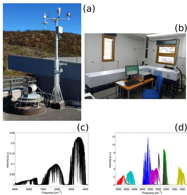
**Fig. 6.** (a) The sun tracker and meteorological station of the FTIR instrument. (b) The high-resolution Bruker IFS 125/HR infrared spectrometer in the room underneath the solar tracker. (c) A near-infrared spectrum collected according to the TCCON specifications on 18 April 2013. (d) Several mid-infrared spectra, collected using different NDACC optical filters and two different detectors (InSb and HgCdTe). These spectra were recorded on 28 May 2013.
