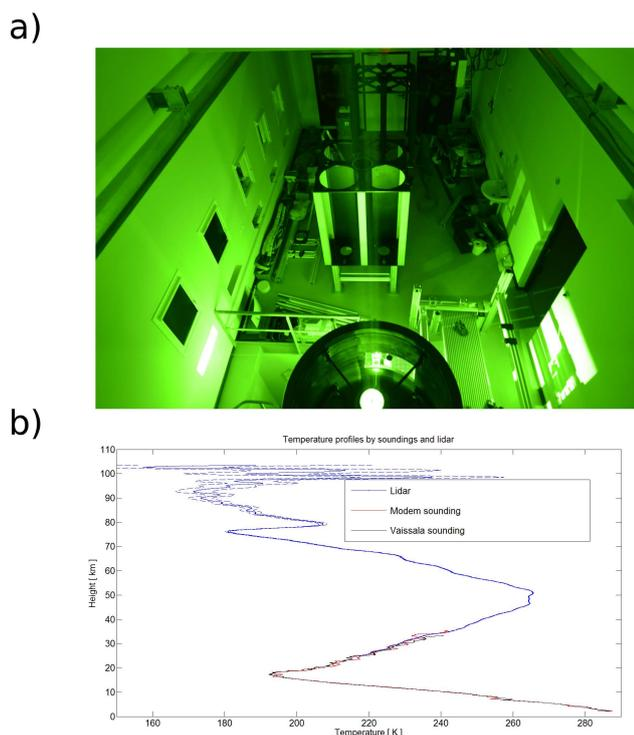
**Fig. 3.** (a) Photo showing the optical reception of the three lidar systems: water vapor and temperature at the foreground, tropospheric ozone at the middle and stratospheric ozone at the background. The lasers are in the room on the left and the spectrometers in the room on the right. (b) Temperature profiles on 2 April 2013 with M10 Modem radiosonde and lidar at Maïdo. Vertical ranges for lidar, Modem and Vaisala Soundings are respectively 24–90 km, 2–35 km and 2–33 km above sea level.
