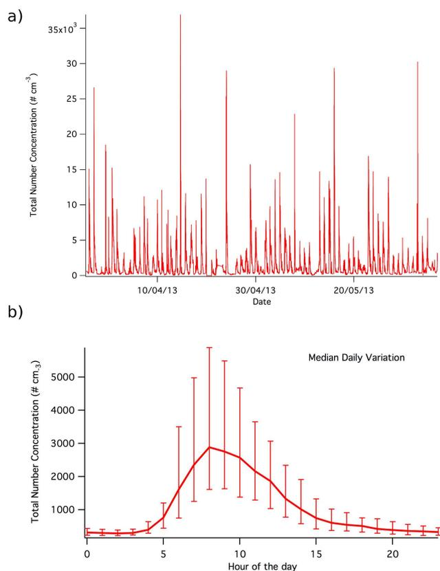
**Fig. 8.** First aerosol total number concentration observed at Maïdo facility: **(a)** 2 months time series (April and May 2013). **(b)** Median daily variation averaged over the whole measurement period.
