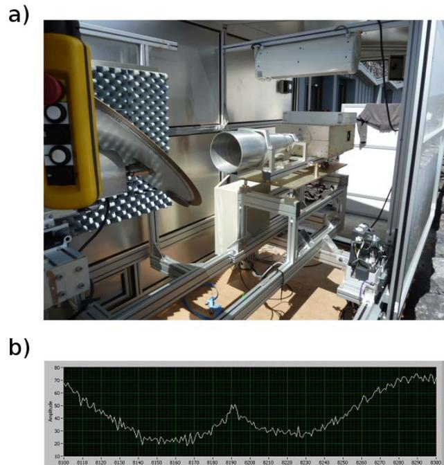
**Fig. 7.** (a) Photo showing the DODO radiometer installed at the Maïdo Observatory in March 2013. (b) Calibrated spectra (Kelvin) obtained on 12 April 2013 at the Maïdo station facility after an integration time of 20 h focusing on the center of the spectrometer ( $\text{H}_2\text{O}$  line center is located at the channel number 8192).
