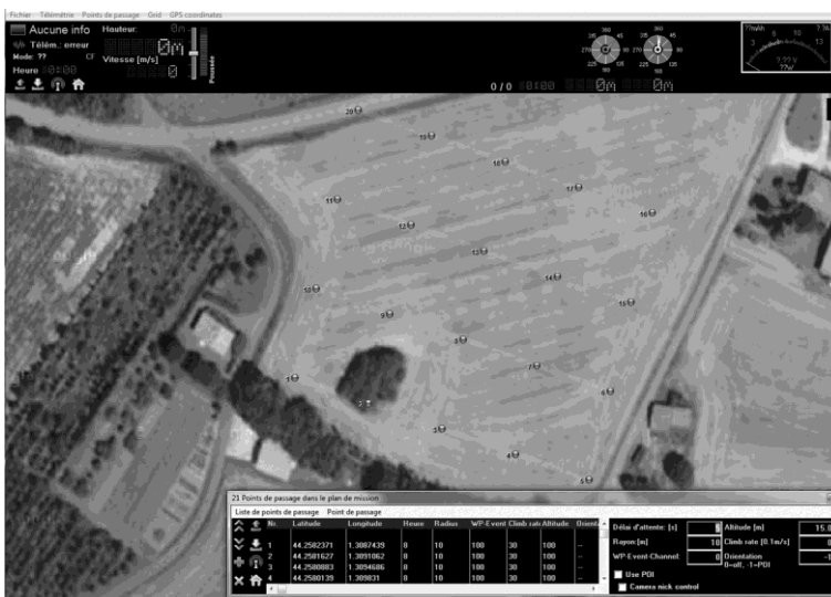
Figure 2 : Definition of a flight plan by equidistant waypoints automatically generated at a plot scale
