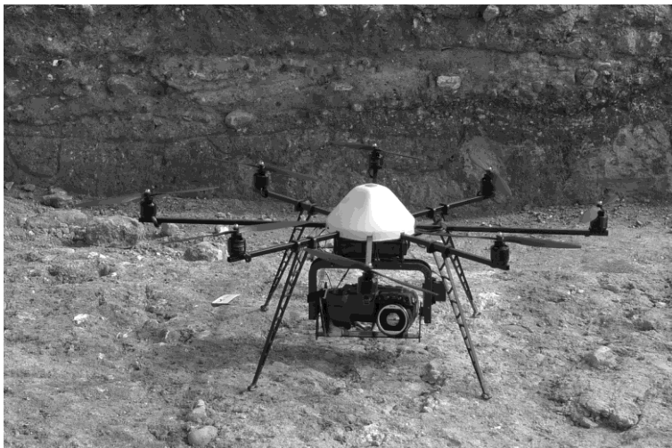
Figure 1 : Drone Octorotor with FLIR T620 thermal camera onboard
