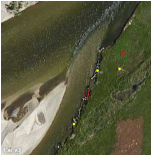
Figure 7: (a) Individual logs and jams within the blue circle on the outside of a meander bend deflecting flow away from the bank and inhibiting lateral channel migration; (b) a collection of individual logs and jams in a favourable position to prevent bank erosion within the blue circle. Red lines indicate individual logs, yellow circles indicate jams, blue circles indicate the area of interest and white arrows point downstream.
