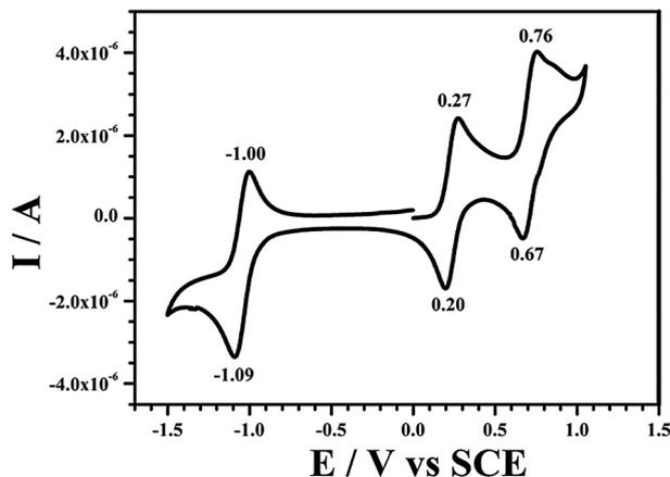
Fig. 7 Cyclic voltammogram at  $0.1 \text{ V s}^{-1}$  of the  $(\text{Cp})_2\text{Ti}(\text{TTF2})$  complex in  $\text{CH}_2\text{Cl}_2\text{-}[\text{NBu}_4][\text{PF}_6]$  0.2 M at 298 K ( $v = 100 \text{ mV s}^{-1}$ ).
