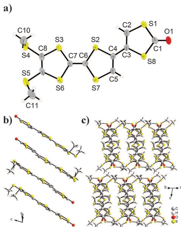
**Fig. 1** (a) Molecular structure of the two crystallographically independent **TTF1** molecules with the atomic numbering (ellipsoids drawn at the 50% probability level); (b) representation of the stacks observed along the [110] direction; (c) projection of the crystalline structure along the [110] direction.
