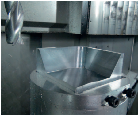
Figure 7: 5-axis machining of the large corner.
