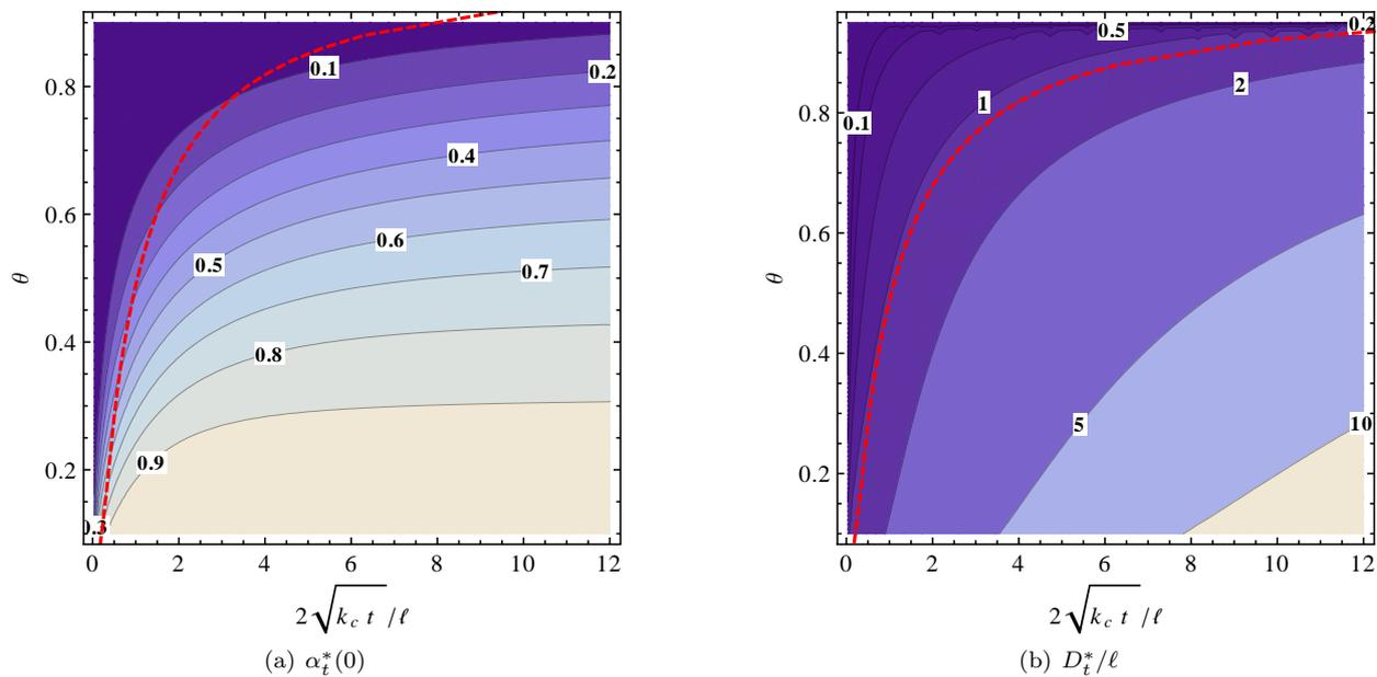
Figure 6: Fundamental solution: damage at the surface  $\alpha_t^*(0)$  and penetration of the damage  $D_t^*$  of the as a function of the thermal shock mildness ( $\theta$ ) and time. The red dashed line indicates the bifurcation time as a function  $\theta$  and separate the parameter space in regions where the fundamental solution is unique or not.
