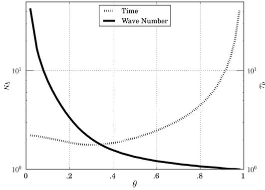
Figure 11: Wave number and rescaled time at the first bifurcation point  $\kappa_b$ ,  $\tau_b$  defined by (57) and (63) for a vanishing Poisson ratio  $\nu = 0$
