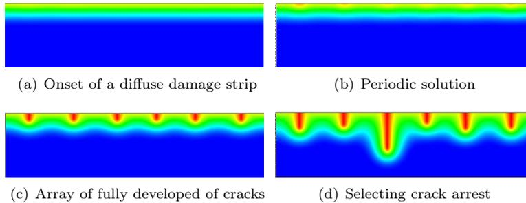
Figure 2: Damage variable  $\alpha$  for four time steps of the minimization process. The loading is given by the thermal shrinking induced by cooling through the top surface. In blue, the sound material; in red, the totally damaged material.
