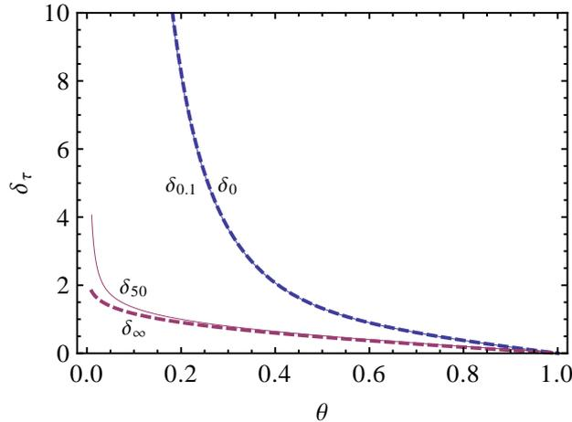
Figure 4: Asymptotic result for the scaled depth of the damage strip  $\delta_\tau$  as a function of the mildness thermal shock  $\theta$ . The dashed lines are the results for  $\tau \rightarrow 0$ ,  $\delta_0$ , and for  $\tau \rightarrow \infty$ ,  $\delta_\infty$ . The continuous lines are the results of the numerical root finding in the shooting method for short ( $\tau = 0.1$ ) and long ( $\tau = 50$ ) times.
