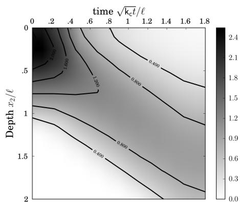
Figure 7: Check of the irreversibility condition: Total time derivative of the damage field of the fundamental branch  $\alpha_t^*$  with respect to time,  $\dot{\alpha}_t^*$ , for the loading  $\theta = .2$ .
