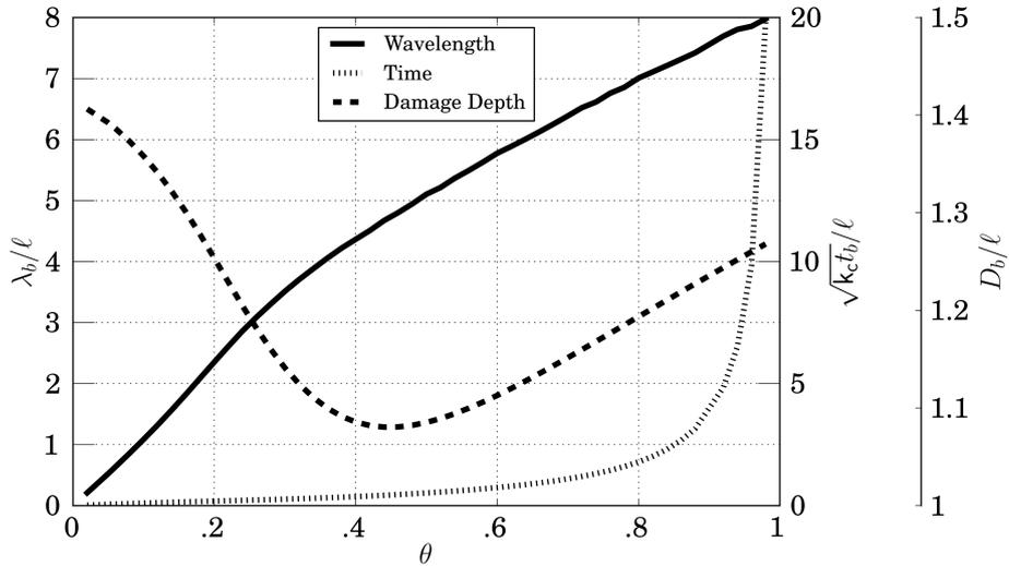
Figure 13: Wavelength  $\lambda_b$ , time  $t_b$  and penetration of the damage zone  $D_b$  at the first possible bifurcation (given by (65), (68)) for a vanishing Poisson ratio  $\nu = 0$  as a function of the loading parameter  $\theta$
