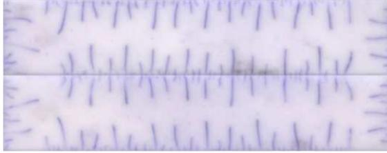
Figure 1: Crack pattern in a slab after a thermal shock (from Jiang et al., 2012)
