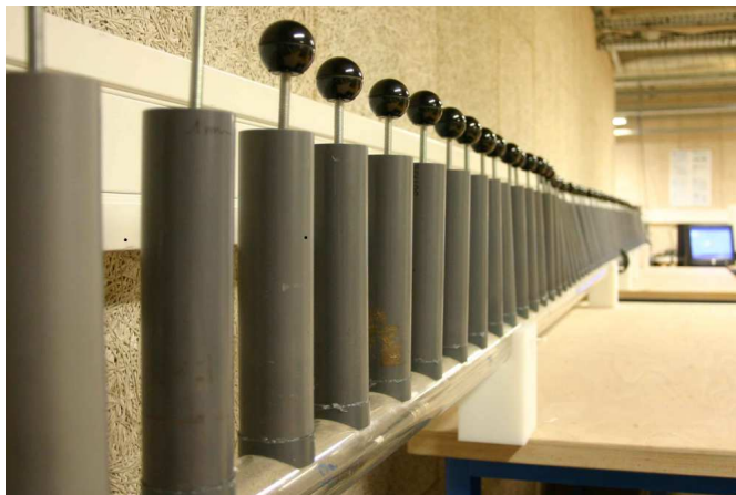
Figure 1: Guide with an array of Helmholtz resonators (courtesy given by O. Richoux).
