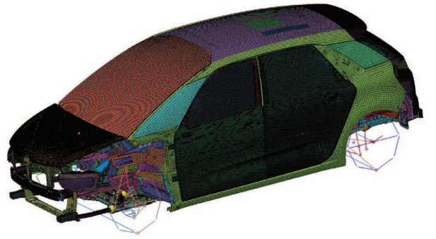
Fig. 3. Finite element computational model of an automobile.
