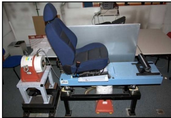
Figure 2: Vibrating test bench
