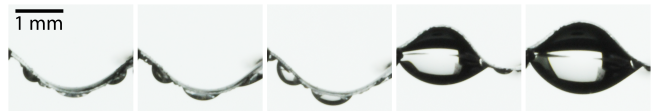
FIG. 5. Condensation-induced snapping. A thin PDMS sample, made hydrophilic on the lower face, is placed in a steam flow. Tiny droplets nucleate on the hydrophilic face and coalesce. When the resulting drop is sufficiently large, elastocapillary snapping takes place. The experiment approximately lasts three minutes.
