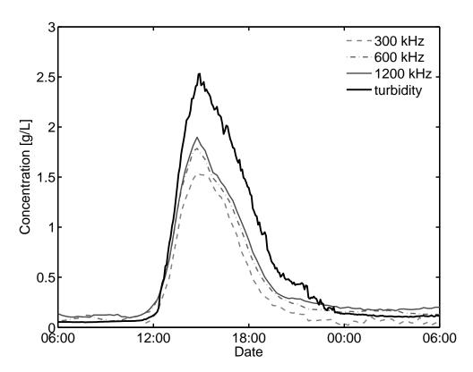
Figure 8 Concentrations measured by the H-ADCPs during Event  $\mathbf{B}$  using the empirical attenuation coefficients calculated from Event  $\mathbf{A}$ , compared to measurements from the optical turbidity meter.
