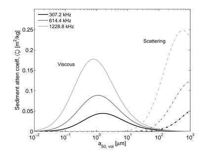
Figure 2 The viscous (–), scattering (-.-) and total attenuation coefficients (...) for a suspension of particles having log-normal distributions by volume with  $\sigma = 1$ , as a function of median radius by volume,  $a_{50 \text{ vol}}$ , for the operating frequencies of the H-ADCPs. The viscous attenuation is calculated assuming spherical particles.
