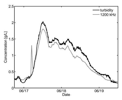
Figure 9 Event **C**: Concentration values measured with the turbidity meter compared to estimates from the 1200 kHz attenuation using the empirical attenuation coefficient from Event **A** in the conversion.
