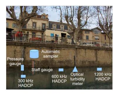
Figure 5 The Romans-sur-Isère study site (Color online). All instruments are installed along the wall of the right bank except the 300 kHz H-ADCP which is attached to a 6-m long arm. To give an idea of scale, the thick vertical bars of the railing are separated by 2 m.
