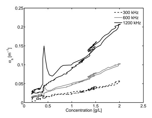
Figure 10 Sediment attenuation measured by the three H-ADCPs as a function of concentration from the turbidity meter for data collected during the flood presented in Figure 9.
