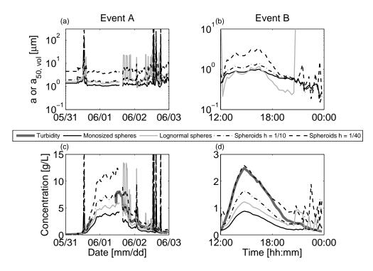
Figure 12 Multi-frequency inversion to grain size (a,b) and then to concentration (c,d) for Events **A** and **B**. For the spheroidal model the radius is the radius of an equal volume sphere. The concentration estimates are obtained by dividing the attenuation observed at 1200 kHz by the theoretical attenuation coefficients for the sizes shown in subplots (a,b).
