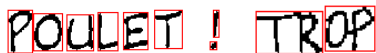
Figure 3: Example of connection between letters. On the left a word with only detached letters, on the right a word detected as two pairs of attached letters because of the handwriting.
