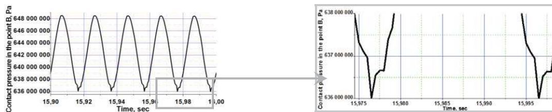
Figure 6. Dependence of the contact pressure over time at the point B at stationary forced vibrations
