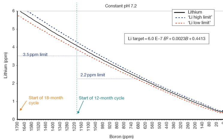
Figure 1.5: Concentration range of boric acid versus lithium hydroxide in order to maintain the  $pH_{300^{\circ}C}$  around 7.2 for different fuel cycle lengths [18].
