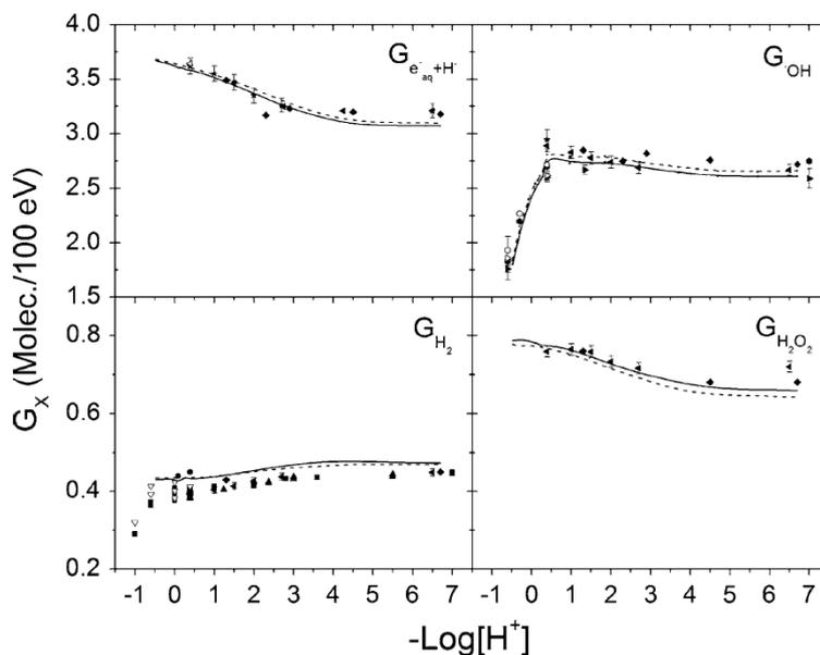
Figure 2.11: Primary yields of  $\text{HO}^\bullet$ ,  $\text{H}_2\text{O}_2$ ,  $\text{H}_2$  and reducing species ( $\text{e}_{\text{aq}}^- + \text{H}^\bullet$ ) versus  $-\text{Log}[\text{H}^+]$  for the radiolysis of air-free aqueous sulfuric solution at  $25^\circ\text{C}$  with 300 MeV protons. Broken line: IONLYS-IRT calculation; solid line: SBS calculation; spline: Monte-Carlo simulation results [32].
