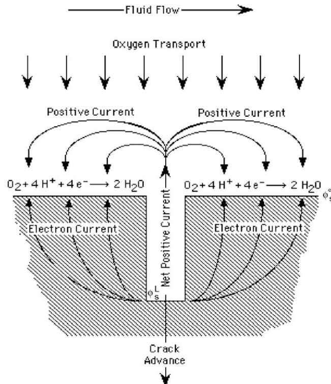
Figure 3.29: Coupling of crack internal and external environments [98].
