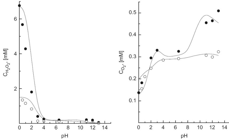
Figure 2.17: The concentration of H<sub>2</sub>O<sub>2</sub> and O<sub>2</sub> versus pH at room temperature under different dose rates: ● = 4.72 Gy.s<sup>-1</sup>; ○ = 0.42 Gy.s<sup>-1</sup> [46, 91].
