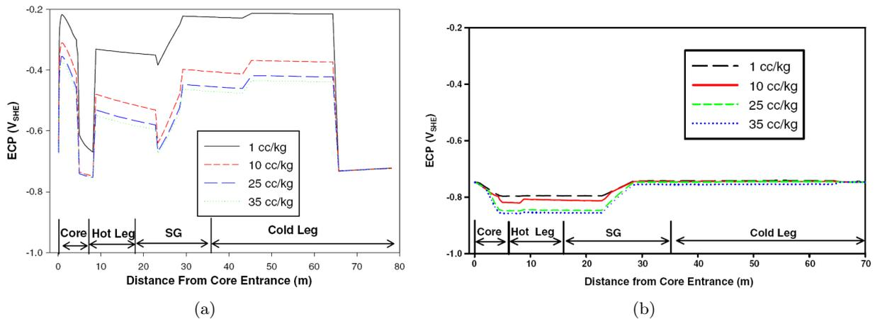
Figure 3.30: Calculated ECP in the primary circuit of a PWR, concentration of  $O_2 = 5$  ppb, concentration of  $H_2$  varied (1, 10, 25, 35 cc/kg): (a) Model uses *high* set of radiolytic yields; (b) Model uses *low* set of radiolytic yields [99].
