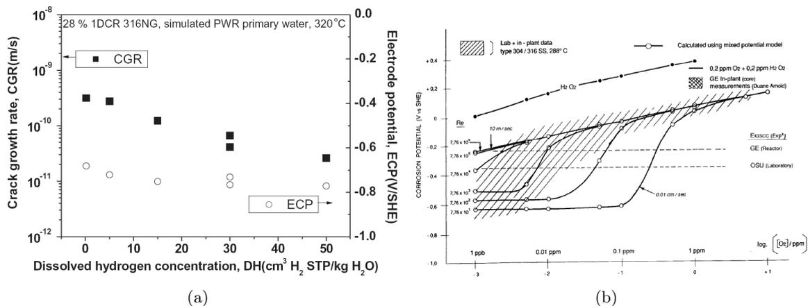
Figure 3.22: Corrosion potential evolution in the presence of  $\text{H}_2$ ,  $\text{O}_2$  and  $\text{H}_2\text{O}_2$ . (a): Crack growth rate (left axe) and electrode potential (right axe) versus dissolved hydrogen for a 316L in a simulated primary PWR water at 320°C [71]; (b): Electrochemical corrosion potential versus the concentration of  $\text{O}_2$  and  $\text{H}_2\text{O}_2$  at 288°C in BWR conditions [72].
