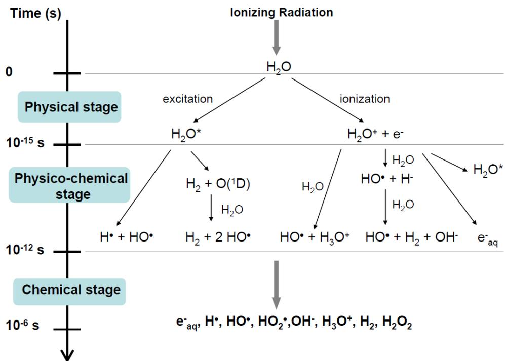
Figure 2.7: Schematic diagrams of water radiolysis [19].
