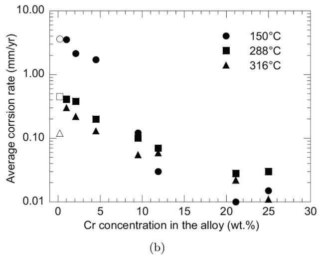
Figure 3.18: The effect of chromium content on the corrosion rate : (a) the parabolic rate constant as a function of Cr% in the alloy under simulated PWR primary condition at 320°C for 380 hours [10]; (b) average corrosion rate of steels as a function of Cr%, in boric acid solution at different temperatures [39].
