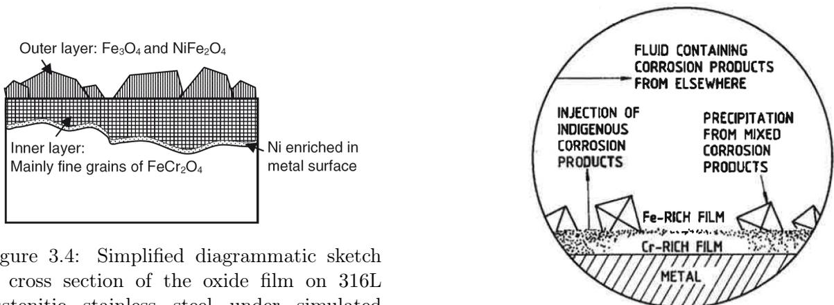
Figure 3.4: Simplified diagrammatic sketch of cross section of the oxide film on 316L austenitic stainless steel under simulated PWR primary water [10].
