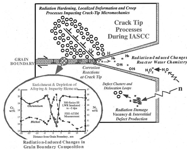
Figure 3.26: Schematic illustrating the different potential parameters on crack advance during IASCC of austenitic stainless steel [90].
