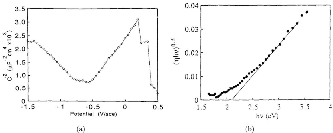
Figure 3.9: Electronic characteristic of the oxide film formed on 316L austenitic stainless steel after 2000 hours exposure at 350°C under a simulated primary PWR environment : (a) Plot of  $1/C^2$  (Mott Schottky plot) as a function of applied potential  $U$ , at 1580 Hz; (b) Plot of  $(\eta h\nu)^{0.5}$  versus the incident light energy  $h\nu$  [7].
