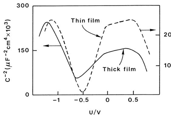
Figure 3.11: Plot of  $1/C^2$  as a function of applied potential  $U$  on stainless steel: a thick passive film formed at high temperature in aqueous environment; a thin passive film formed at 0.6 V/SCE in borate buffer solution at room temperature [13].
