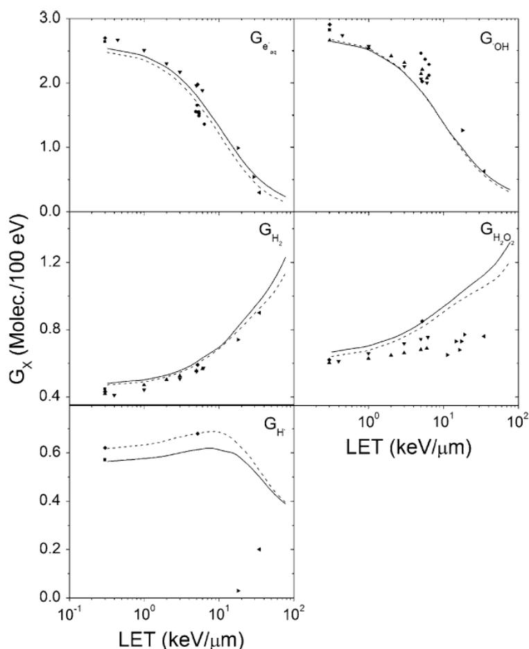
Figure 2.9: Primary yields of  $\text{H}^\bullet$ ,  $\text{HO}^\bullet$ ,  $\text{H}_2$ ,  $\text{H}_2\text{O}_2$  and  $\text{e}_{aq}^-$  in neutral liquid water irradiated by proton (300-0.1 MeV,  $\text{LET} \sim 0.3\text{-}85 \text{ keV}/\mu\text{m}$ ) at  $25^\circ\text{C}$ . Broken line: IONLYS-IRT calculation; solid line: SBS calculation; spline: Monte-Carlo simulation results [32].
