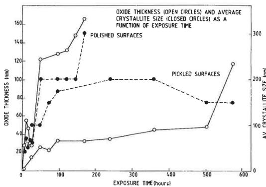
Figure 3.7: Oxide thickness ( $\circ$ ) and average crystallite size ( $\bullet$ ) as a function of exposure time: upper zone polished surface; lower zone pickled zone [4].
