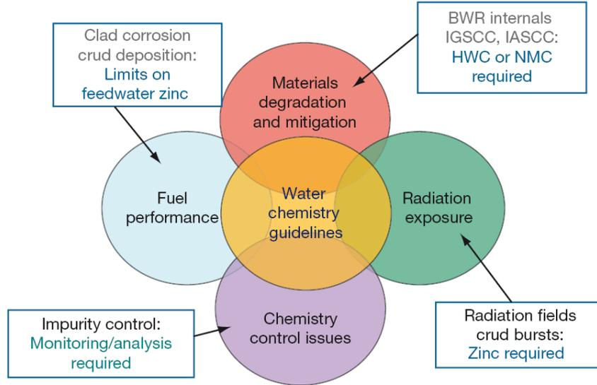
Figure 1.3: Boiling water reactors (BWRs) chemistry interactions. [18]
