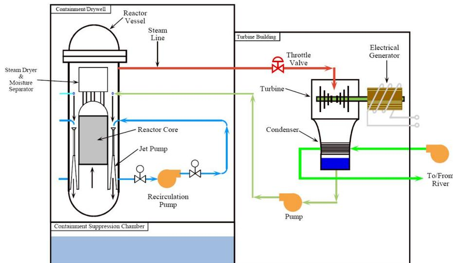
Figure 1.2: Scheme of Boiling Water Reactors (BWRs). [17]
