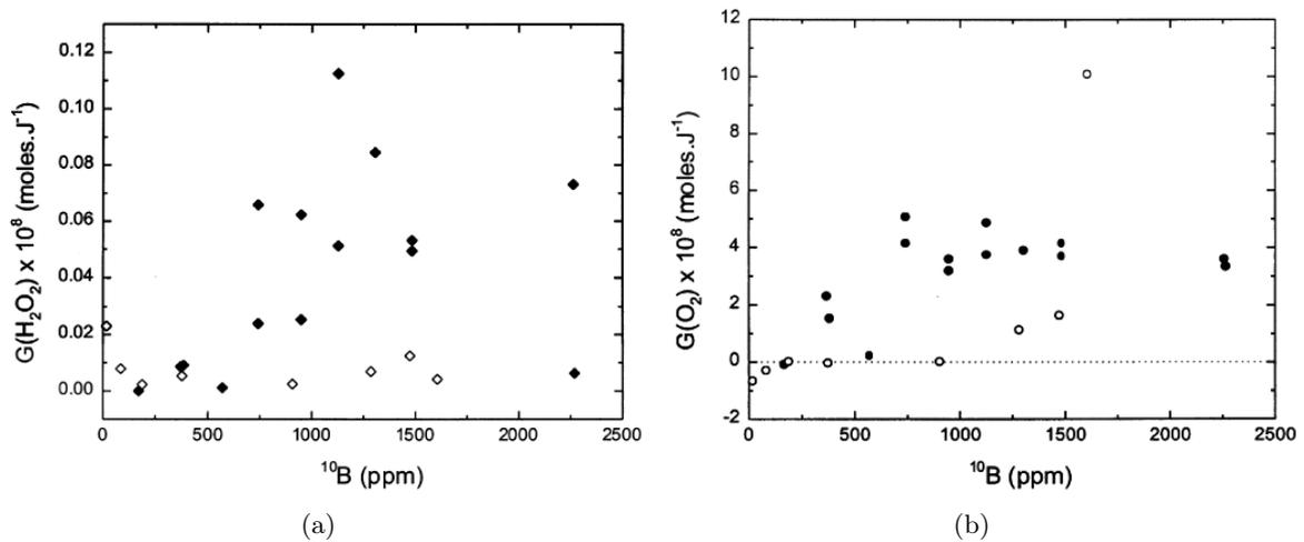
Figure 2.15: The effect of  $^7\text{LiOH}$  on water radiolysis at  $200^\circ\text{C}$ : (a)  $g(\text{H}_2\text{O}_2)$  vs.  $[\text{}^{10}\text{B}]$ ; (b)  $g(\text{O}_2)$  vs.  $[\text{}^{10}\text{B}]$ . Solid symbols: solution contains  $^7\text{LiOH}$ , calculated by MULTEQ<sup>®</sup> to achieve a  $\text{pH} = 7$  at  $200^\circ\text{C}$ ; Open symbols: blank solution without  $^7\text{LiOH}$  [87].
