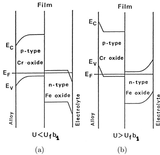
Figure 3.10: Schematic sketch of the electronic structure model of oxide film formed on 316L: (a)  $U < U_{FB} (\approx -0.5 \text{ V})$ ; (b)  $U > U_{FB} (\approx -0.5 \text{ V})$  [13].
