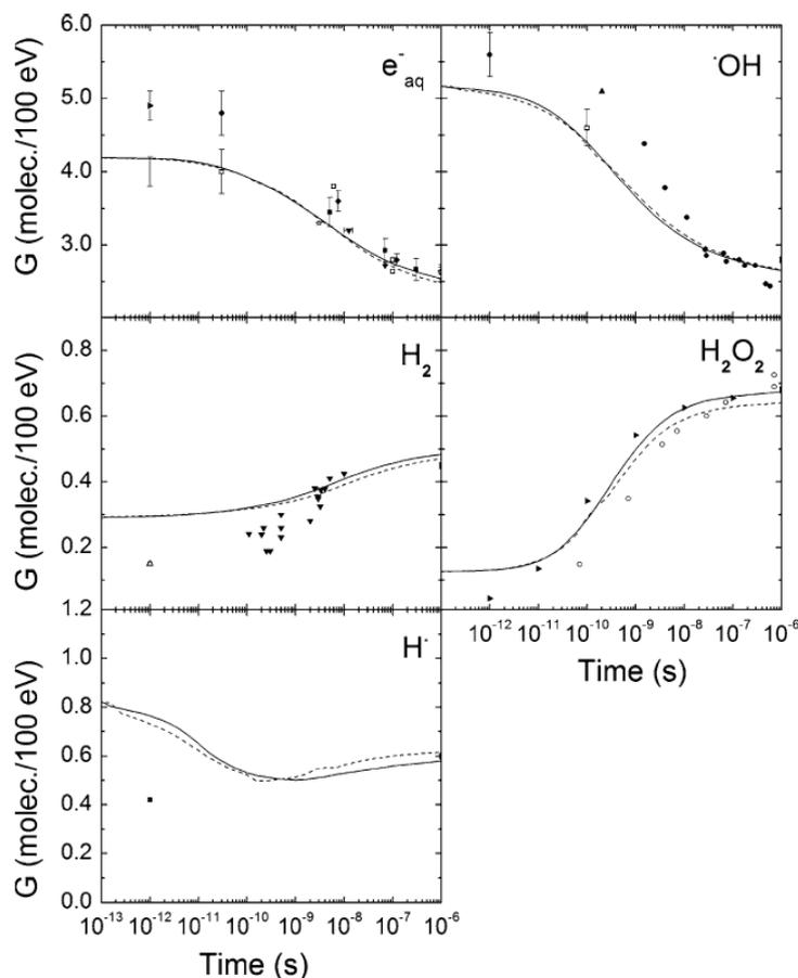
Figure 2.8: Time-dependent of primary yields;  $H^\bullet$ ,  $HO^\bullet$ ,  $H_2$ ,  $H_2O_2$  and  $e_{aq}^-$  produced by low LET radiation tracks of proton (300 MeV, LET  $\sim 0.3$  keV/ $\mu$ m) at neutral pH and 25°C. Broken line: IONLYS-IRT calculation; solid line: SBS calculation; spline: Monte-Carlo simulation results [32].
