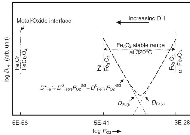
Figure 3.21: Diffusion rate of Fe in spinel oxide versus oxygen partial pressure, calculated for metal/oxide and oxide/oxide interfaces at 320°C [10].
