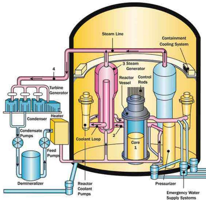
Figure 1.4: Schema of Pressurised Water Reactor.
