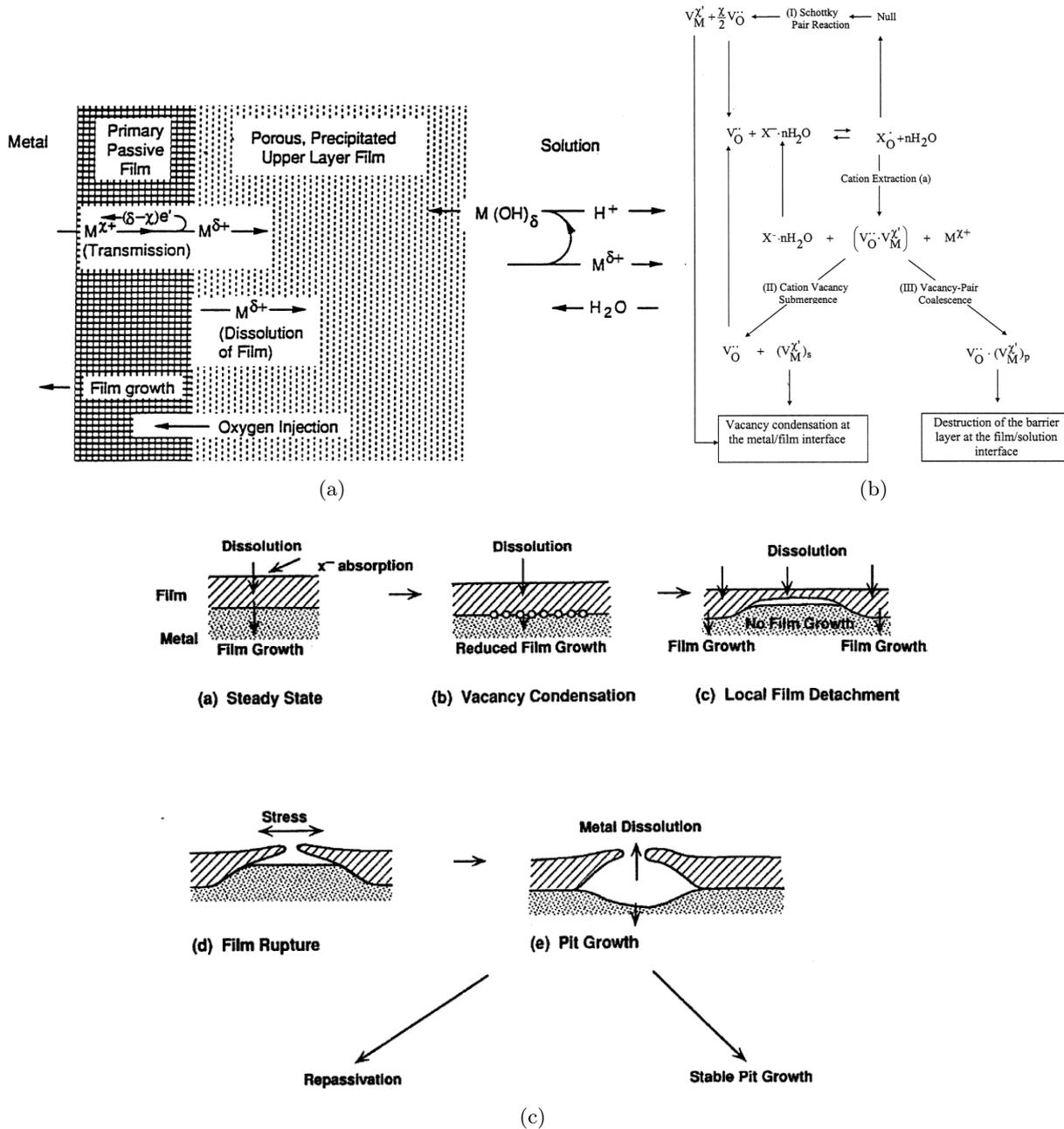
Figure 3.6: Schematic sketch of **Point Defect Model**: (a) process of bilayer passive film formation on the metal surfaces; (b) proposed reactions leading to cation vacancy condensation at the metal/film, film/solution interfaces and eventually the passivity breakdown; (c) cartoon outlining various stages of pit nucleation according to the PDM [27].
