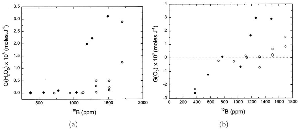
Figure 2.18: The effect of  $Fe(NO_3)_3$  at 30°C on water radiolysis: (a)  $G(H_2O_2)$  vs.  $[^{10}B]$ ; (b)  $G(O_2)$  vs.  $[^{10}B]$ . Solid points: ● and ◆ for 2ppm  $Fe(NO_3)_3$ ; open points: ○ and ◇ for blank solution [87].
