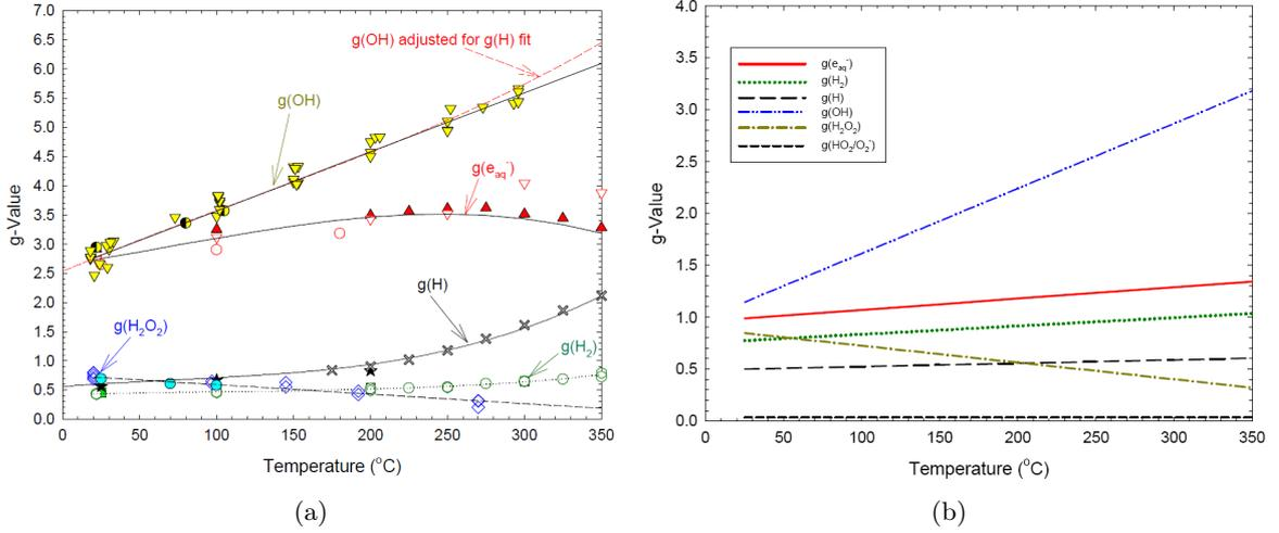
Figure 2.12: The g-values for the primary species formed in reaction 2.18 as a function of temperature: (a) low LET radiation; (b) high LET radiation (fast neutron radiation for natural uranium fuel). [52].
