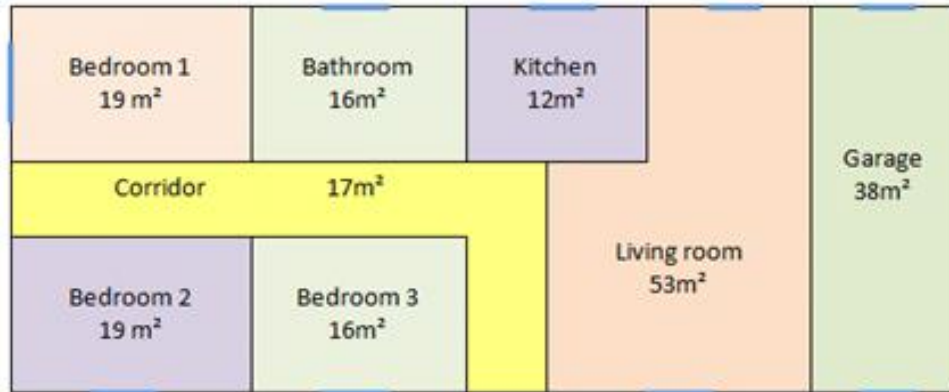
Fig.2. Plan of the 150 m 2 single-storey house. The house features a living room, a kitchen, three bedrooms, a bathroom, a corridor and a garage. Windows are represented in blue
